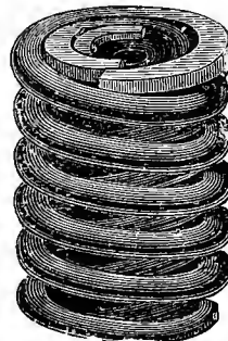
Fig. 5250. ROUND-BAR TRIPLE-COIL SPIRAL-SPRING OR NEST-SPRING.
